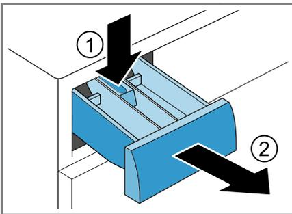
3. Pull out the insert upwards.
